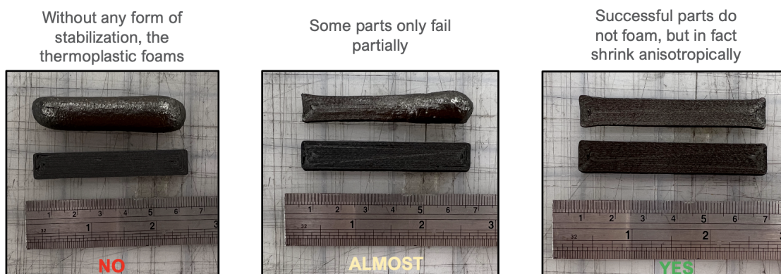
Figure 4.5: Pyrolyzed samples (top) with polymer samples (bottom) of failed sample (left), partially failed sample (center) and successful sample (right).
