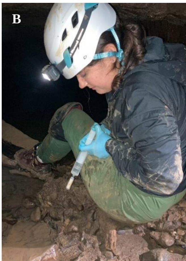
Figure 3.2. (A) Sampling dissolved nitrate inside one of the study caves by using a CHEMetrics field spectrophotometer and colorimetric kit, and (B) filtering water through a Sterivex filter to obtain an eDNA sample (right).
