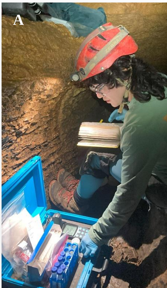
Figure 3.2. (A) Sampling dissolved nitrate inside one of the study caves by using a CHEMetrics field spectrophotometer and colorimetric kit, and (B) filtering water through a Sterivex filter to obtain an eDNA sample (right).
