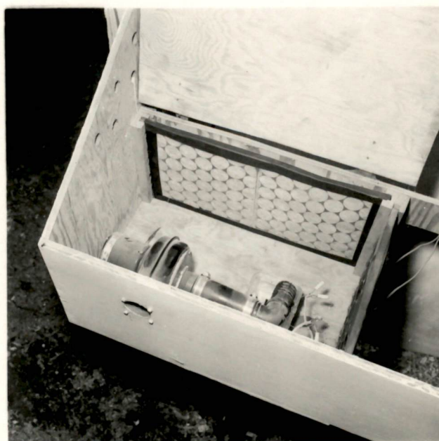
Figure 18. View of outside installation of filter box with cover open.
