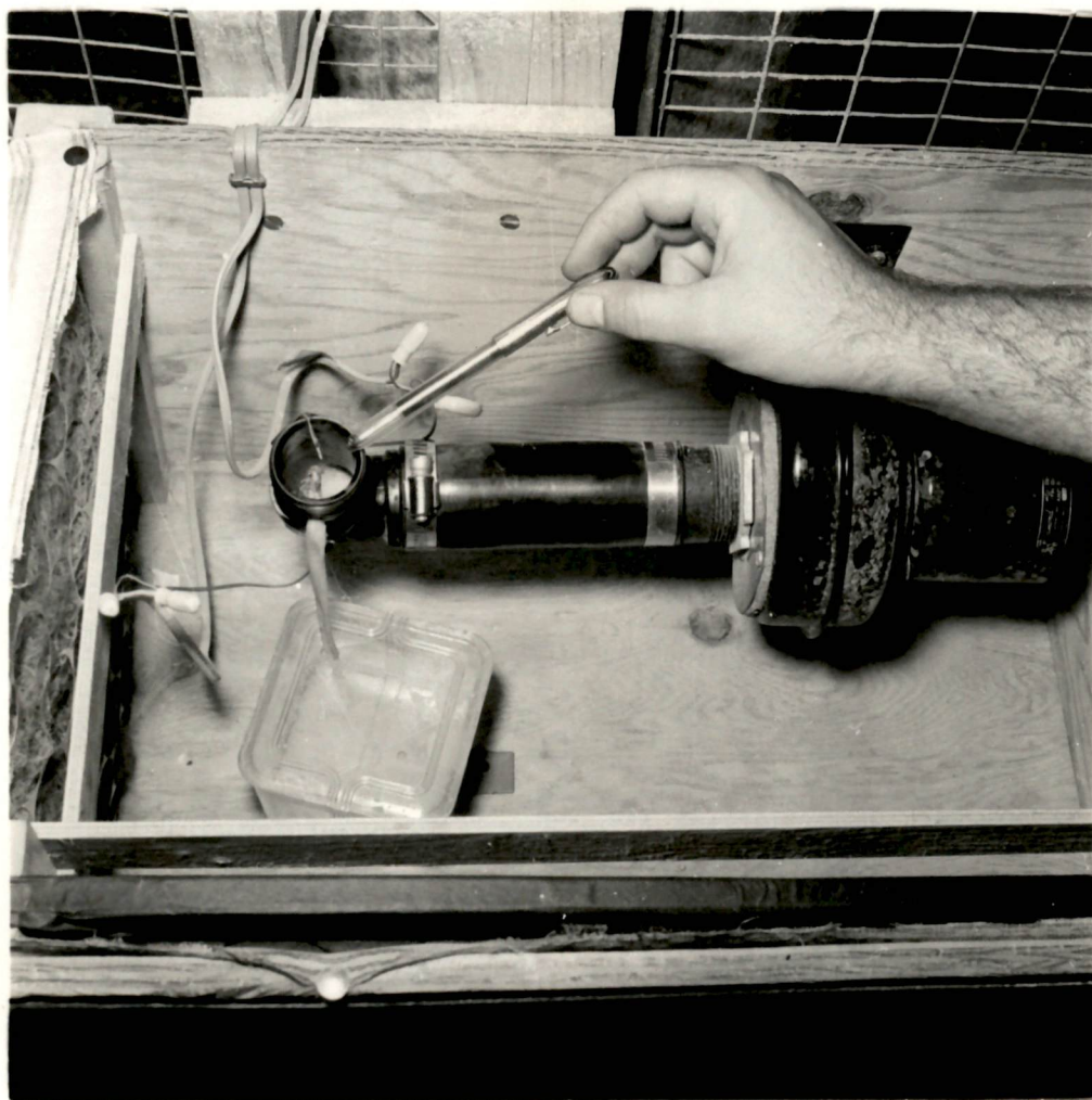
Figure 15. A view of the fan unit showing how the thermocouples were mounted (note wet-bulb wick and container for water).
