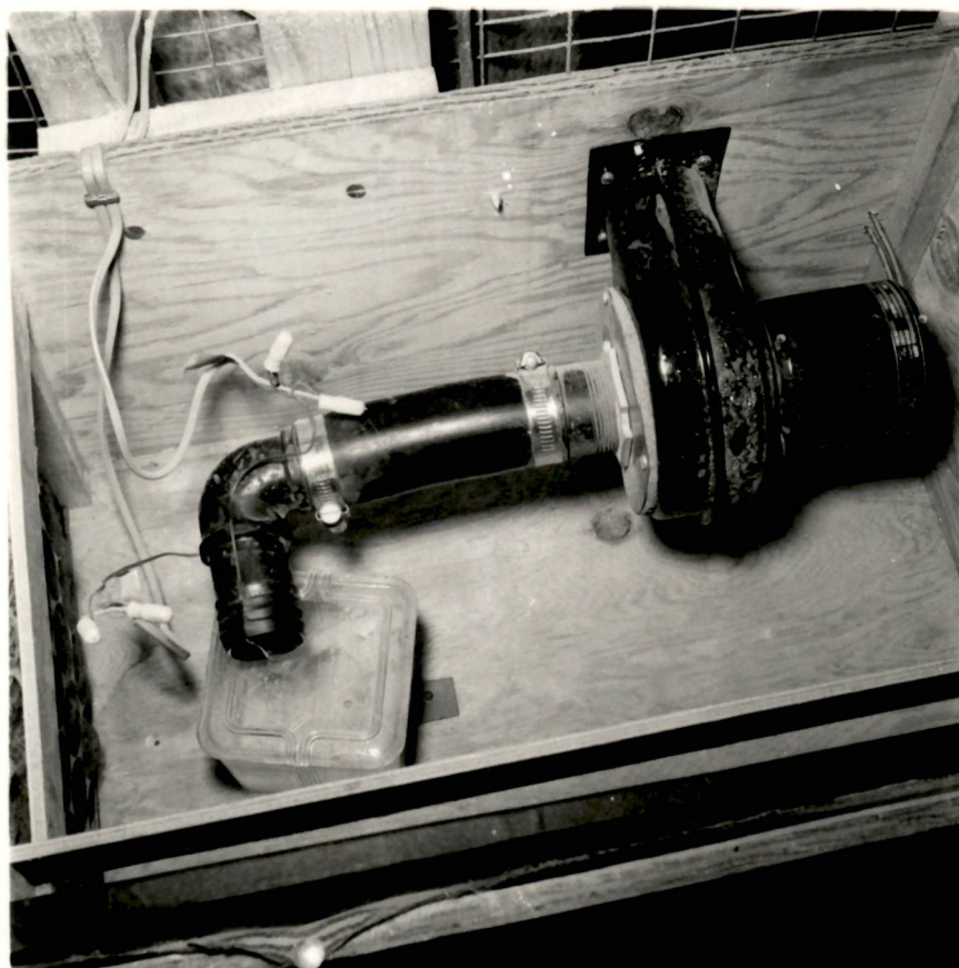
Figure 14. The fan unit used to obtain the air velocity across the thermocouples (note how the plastic pipe is fastened to the fan housing).
