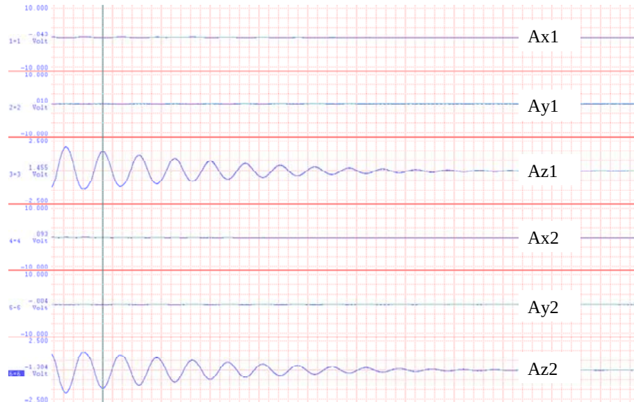
Figure 37: Beam vibration measurement with both accelerometer to test synchronization, cross talk and proper orientation of the axis
