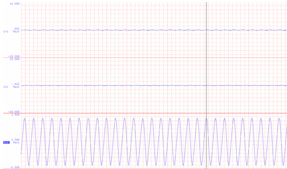
Figure 38: Signal generated from the calibrator and recorded by the accelerometer
