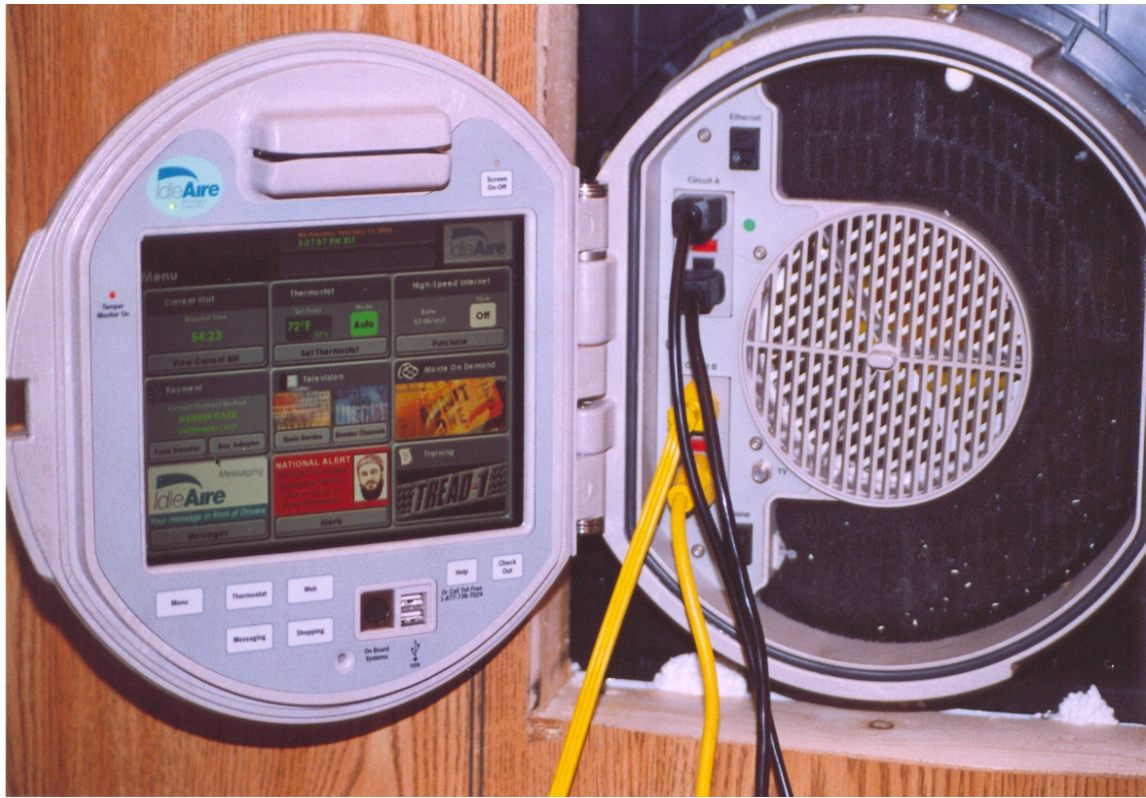
Figure 1.2 IdleAire Electrification Unit Computer Touch Screen and Air Supply
