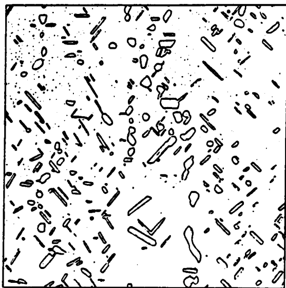
23a. Ni-Ta-Cr alloy, 1250°C, 7 days, water quenched, then reheated to 1280°C for 4 hrs, water quenched, OM, 200 X.
