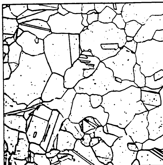
20b. Ni-Ta alloy, aged at 800°C for 500 hrs, water quenched, OM, 100X.
