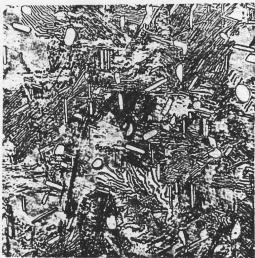
25a. Ni-Ta-Cr alloy, aged at 700°C for 500 hrs, water quenched, 0M, 200 X.
