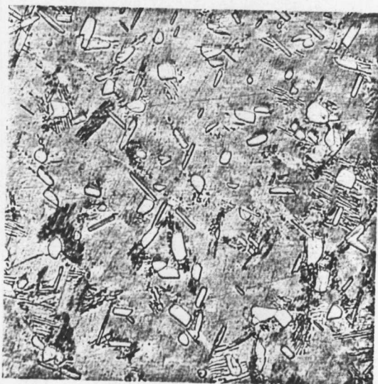
24a. Ni-Ta-Cr alloy, aged at 700°C for 100 hrs, water quenched, OM, 200 X.
