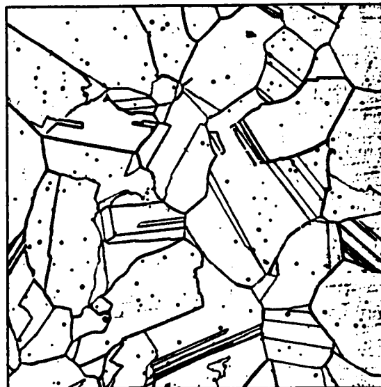
21b. Ni-Ta alloy, aged at 800°C for 1000 hrs, water quenched, OM, 100X.
