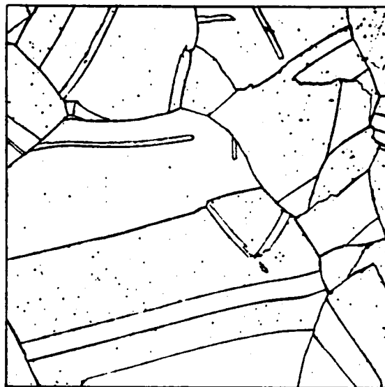
18d. Ni-Ta alloy, aged at 600°C for 1000 hrs, water quenched, OM, 100 X.
