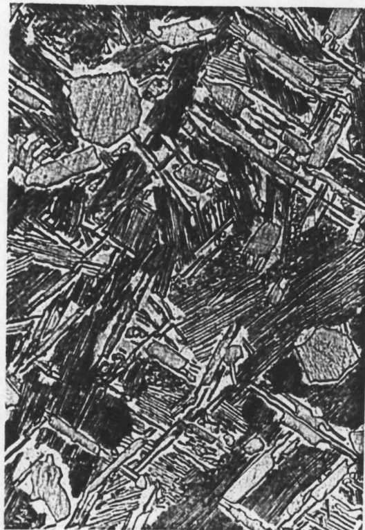
26b. Ni-Ta-Cr alloy, aged at 1000°C for 500 hrs, water quenched, OM, 500 X.
