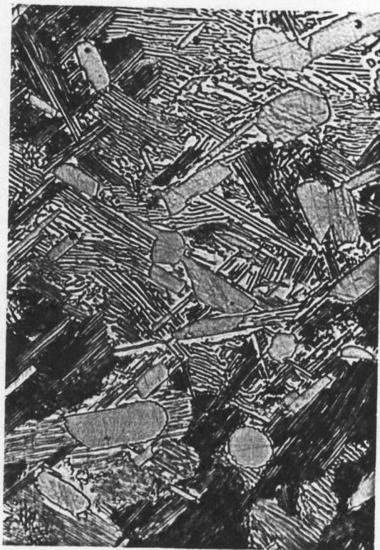
26a. Ni-Ta-Cr alloy, aged at 900°C for 500 hrs, water quenched, OM, 500 X.
