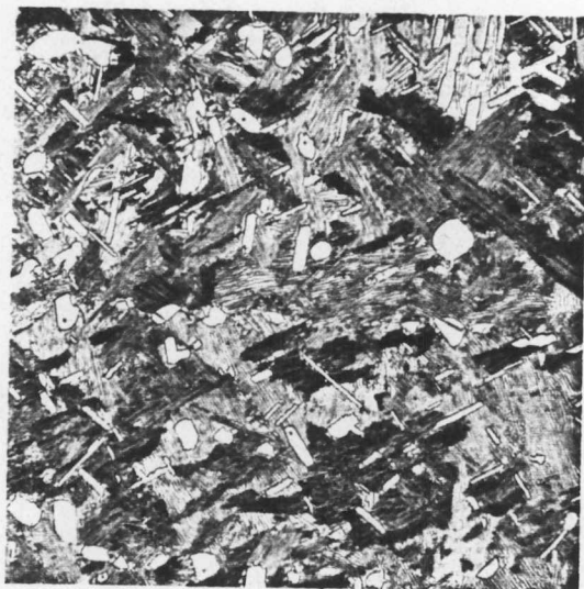
24c. Ni-Ta-Cr alloy, aged at 900°C for 100 hrs, water quenched, OM, 200 X.
