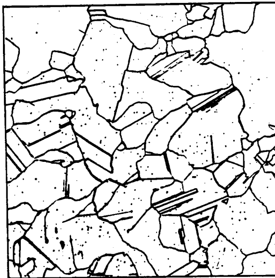
19b. Ni-Ta alloy, aged at 800°C for 100 hrs, water quenched, OM, 100X.
