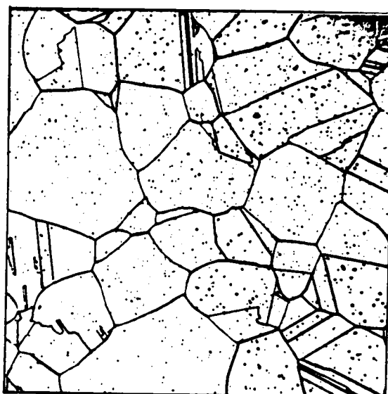
20d. Ni-Ta alloy, aged at 1000°C for 500 hrs, water quenched, OM, 100X.
