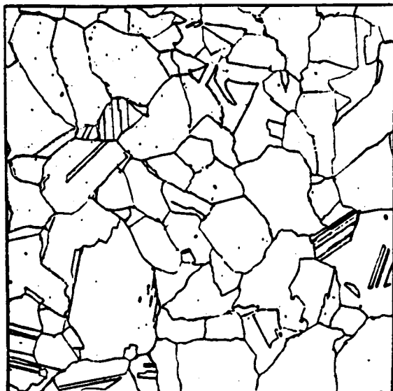
19a. Ni-Ta alloy, aged at 700°C for 100 hrs, water quenched, OM, 100 X.
