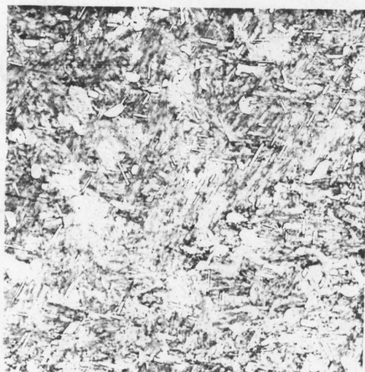
25b. Ni-Ta-Cr alloy, aged at 800°C for 500 hrs, water quenched, 0M, 200 X.
