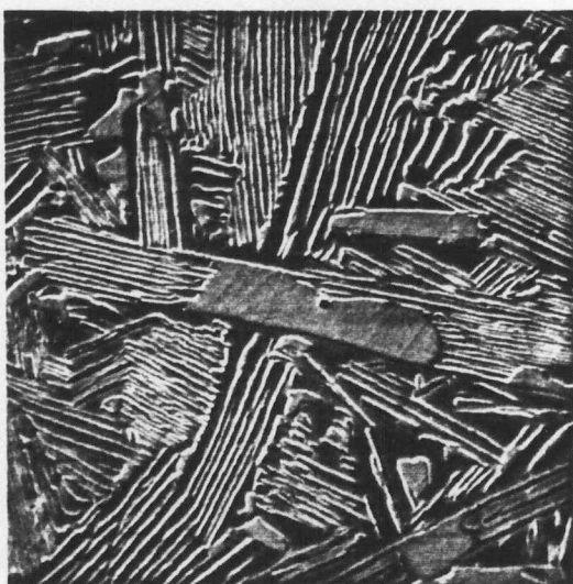
41c. Ni-Ta-Cr alloy, aged at 900°C, 500 hrs, then water quenched, SEM, 2000 X.
