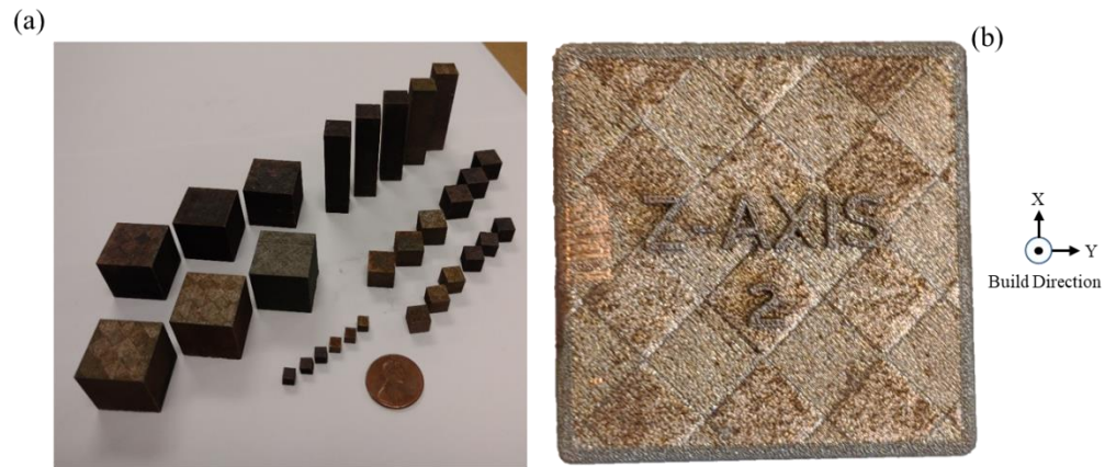
Figure 1.2. L-PBF GRCop-84 samples built on a Concept Laser M2 (a) 4, 7, 10, and 20 mm cubes and 10x10x40 mm pillars and (b) top of a 20 mm cube.
