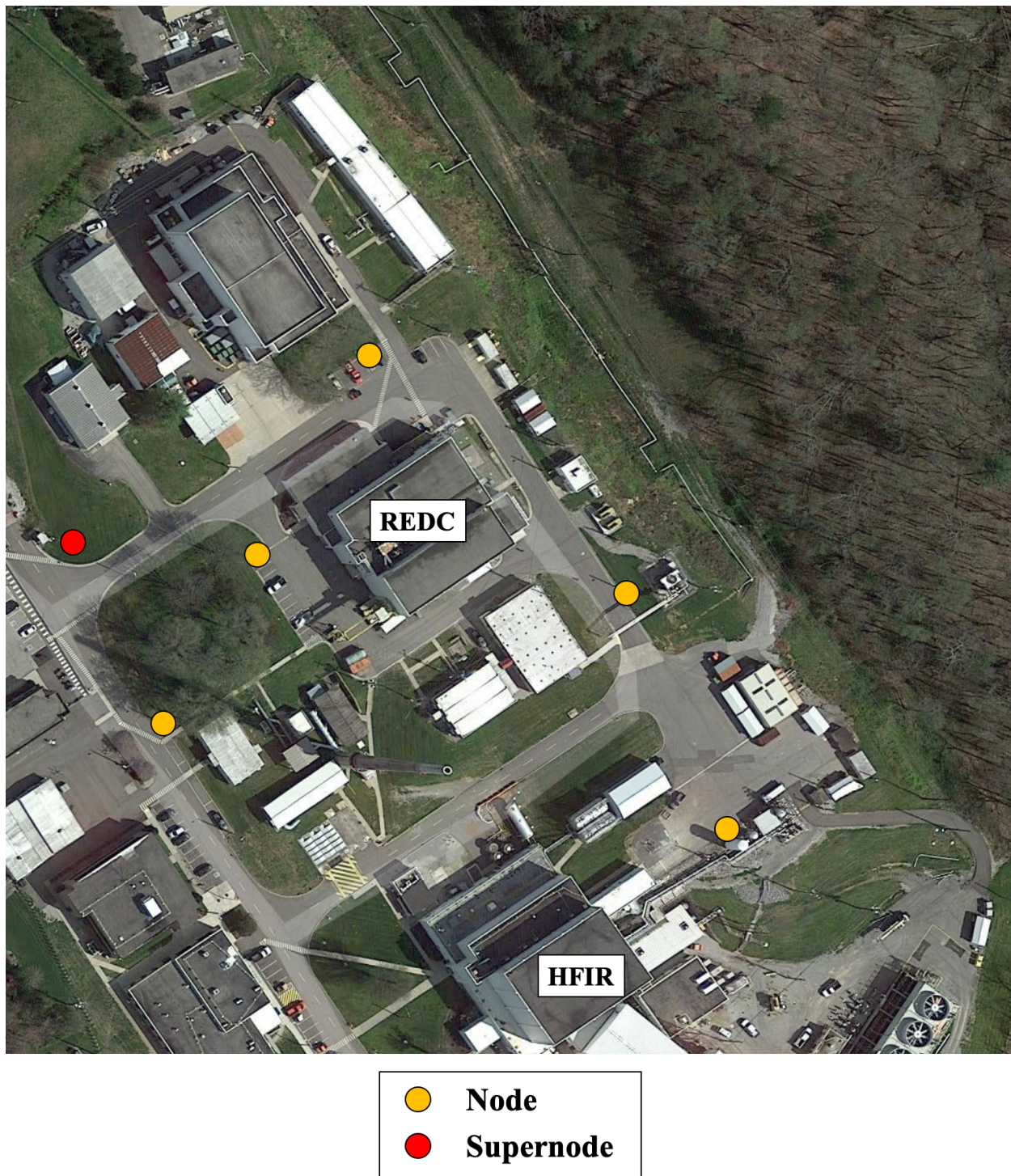
Figure 3.6: Layout of the sensor nodes at the HFIR/REDC facility.
