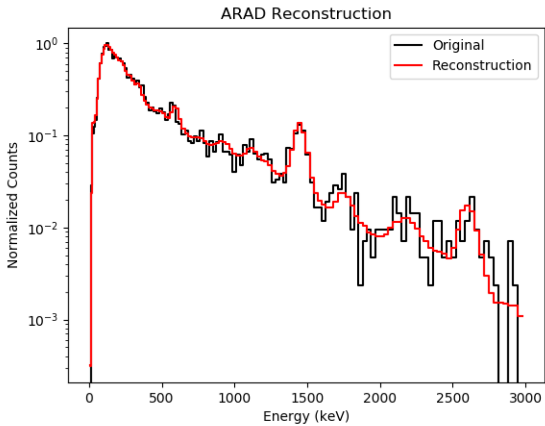
Figure 6.4: Reconstruction of a gamma ray spectrum by ARAD for the precipitation event shown in Figure 6.5. Node 01.
