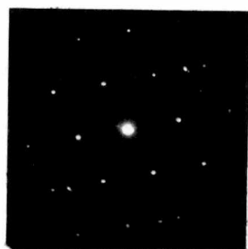
Figure 3.21 Microstructure of a ZnSe film grown by PLD in a 1000 mtorr He/Cl 2 atmosphere. E_d=1.9\text{J}/\text{cm}^2 , r_g=15 sccm. a) overall microstructure b) \langle 110 \rangle electron diffraction pattern of the entire film thickness c) \langle 110 \rangle electron diffraction pattern of the columnar grain region only.
