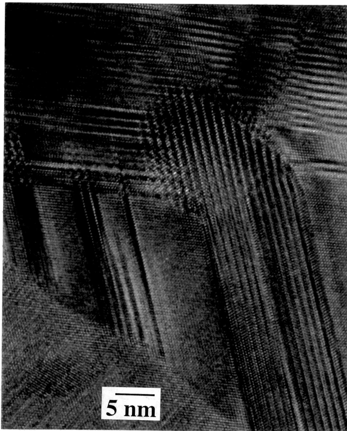
Figure 3.15 Complex of stacking faults in the bulk of the ZnTe film shown in Figure 3.14.
