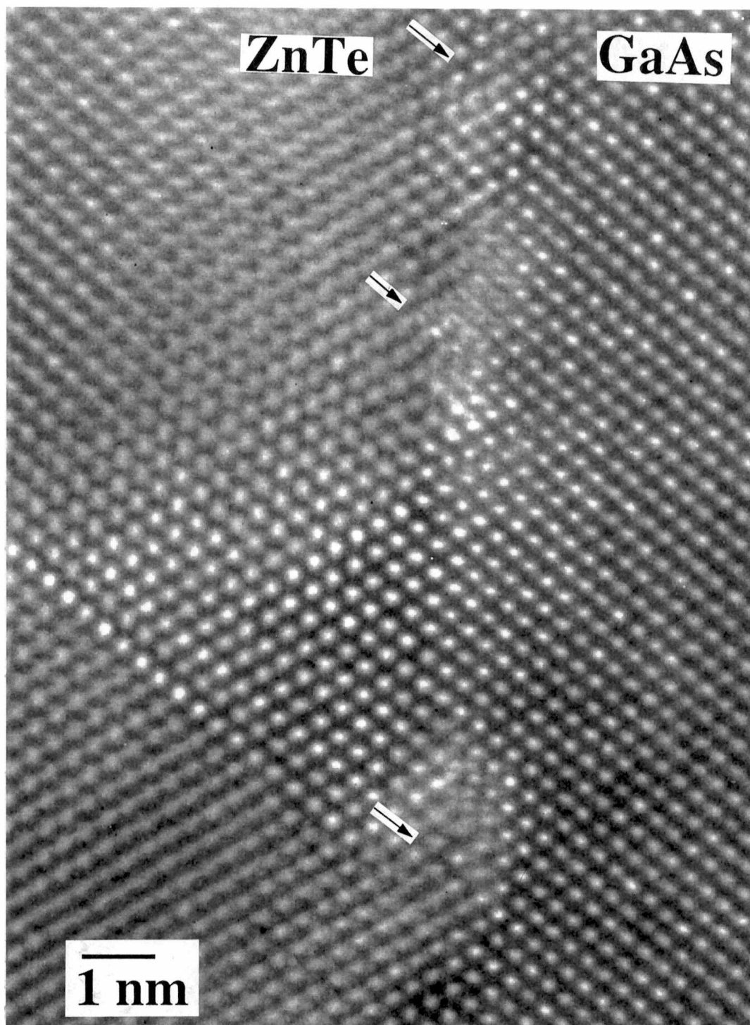
Figure 3.28 Misfit dislocations (arrows) along the interface of the undoped ZnTe/GaAs film grown by MBE shown in Figure 3.1.
