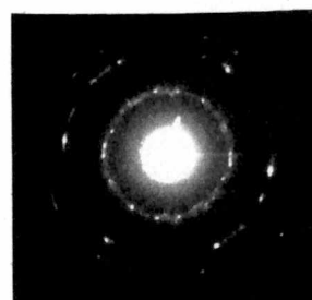
Figure 3.21 Microstructure of a ZnSe film grown by PLD in a 1000 mtorr He/Cl 2 atmosphere. E_d=1.9\text{J}/\text{cm}^2 , r_g=15 sccm. a) overall microstructure b) \langle 110 \rangle electron diffraction pattern of the entire film thickness c) \langle 110 \rangle electron diffraction pattern of the columnar grain region only.
