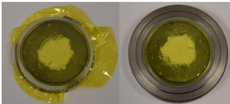
Figure 10: Powder XRD sample holder without (left) and with (right) outer sample holder with NaI powder loaded.
