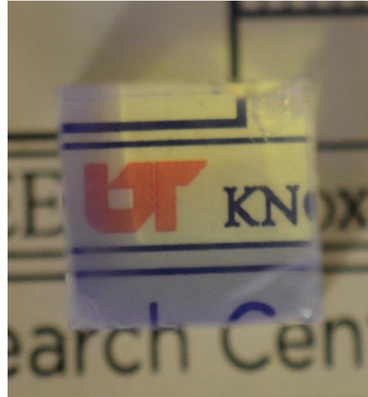
Figure 25: Full boule of \text{CsCaBr}_{0.8}\text{I}_{2.2}:\text{Eu} 2% (left) and a 1 cm cube sourced from the crystal.
