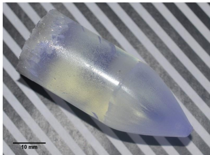
Figure 28: Ø22 mm CsCaBr 0.8 I 2.2 :Eu crystal as removed from the growth ampoule. The rough surface texture is easily polished away.
