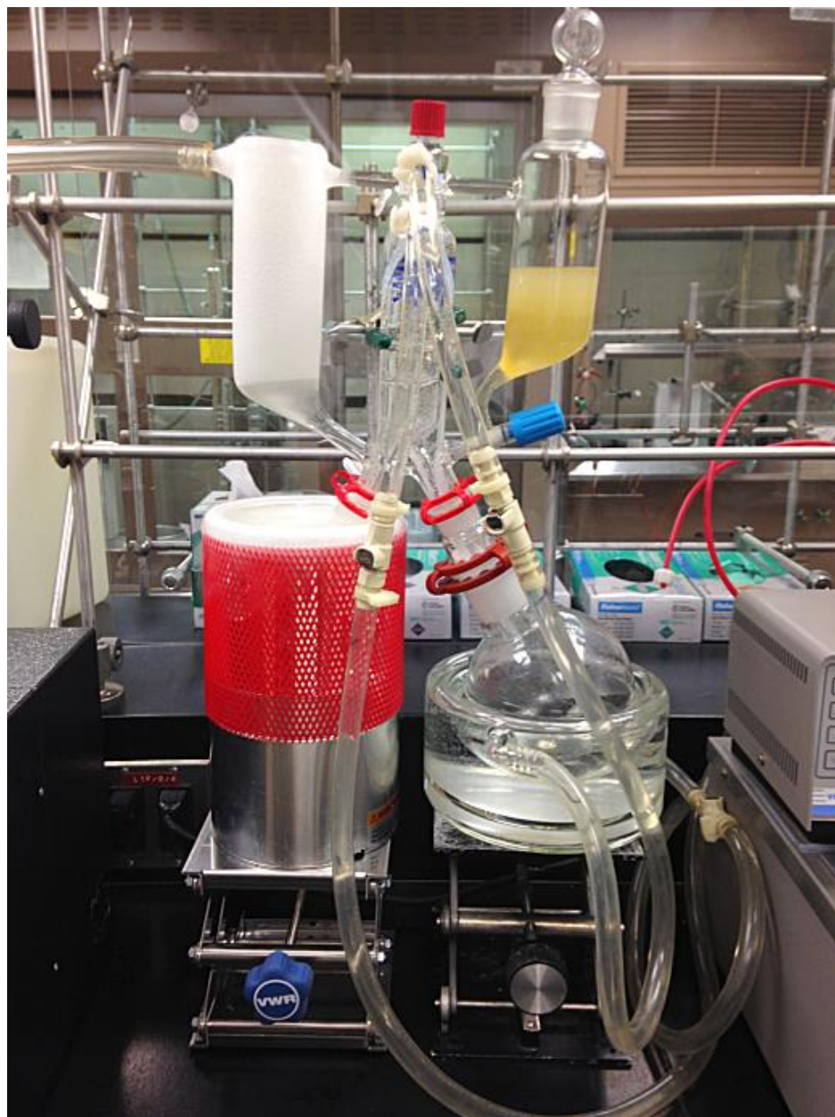
Figure 8: Solvent Assisted Flavor Evaporation (SAFE) apparatus in use
