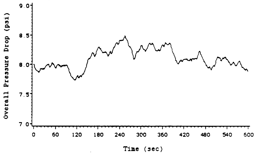
Figure 4.5: Integrated Autoregressive (IAR) Disturbance
