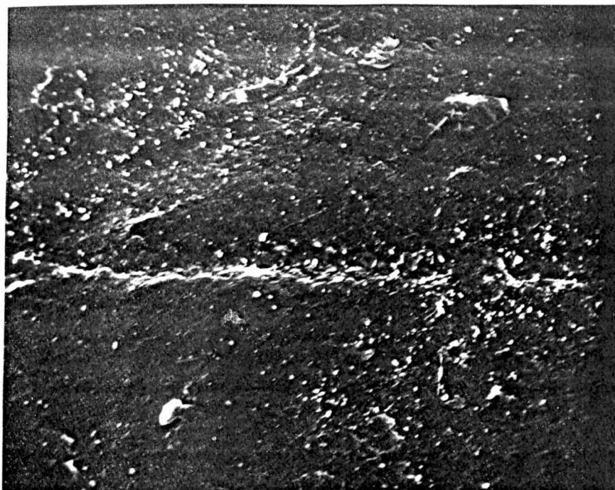
(A) With weld line (in center).
