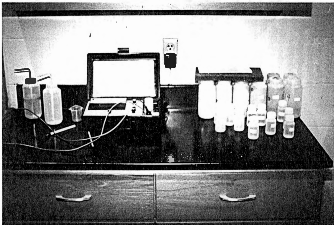
Figure 7. Field conductivity meter for measuring chemical concentration in the nozzle effluent.
