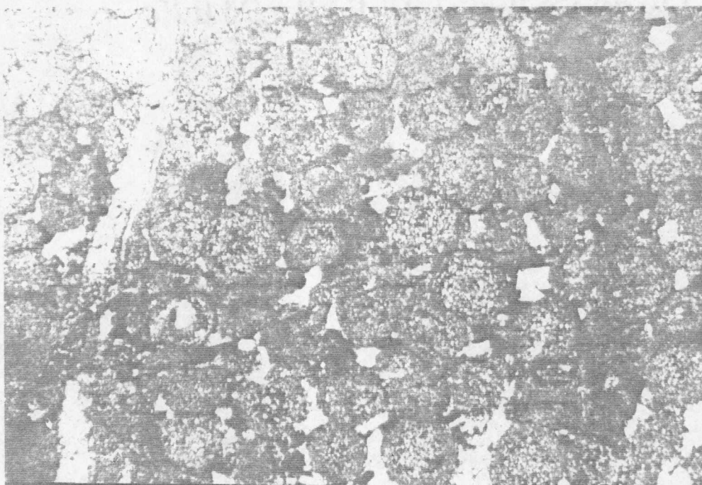
Figure 32. Calcite Filled Bedding Normal Extension Fractures in the Rome Oolite. Field of view is 3.2 mm by 2.15 mm.
