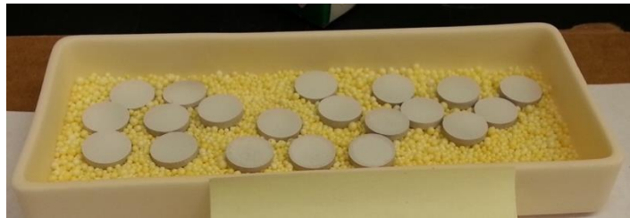
Figure 3.2 Thin \text{Gd}_2\text{Ti}_2\text{O}_7 pellets inside zirconia boat before 2 nd sintering.
