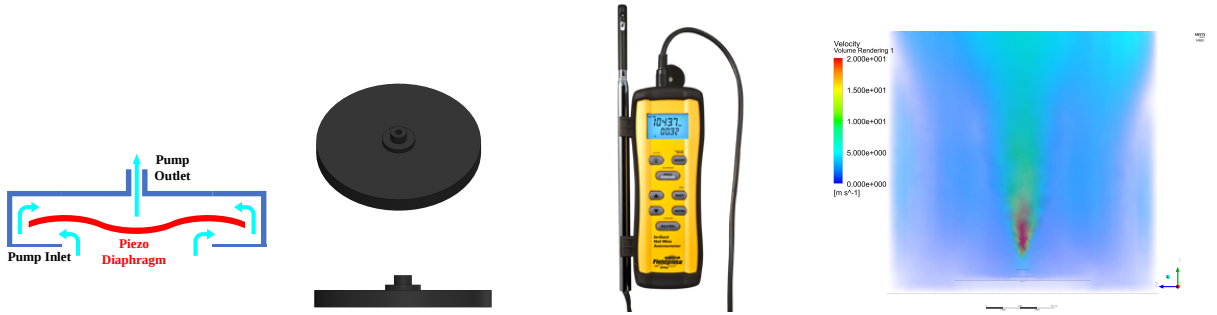
Figure 5.5: Micro piezo-electric pump (a) Micro pump actuation concept. (b) Pump design and dimensions. (c) Pump analysis setup: Anemometer used for measuring the immediate velocity of pump outlet.
