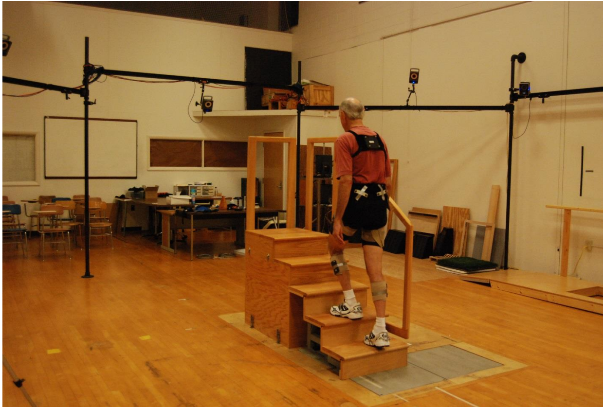
Figure 1. The staircase with the instrumented steps (steps 1-3) and non-instrumented steps (steps 4-5) for continuous motion with a landing platform.
