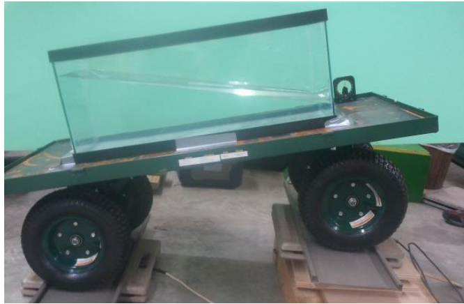
Figure 4.7. Model validation with a wagon that carries a liquid tank.
