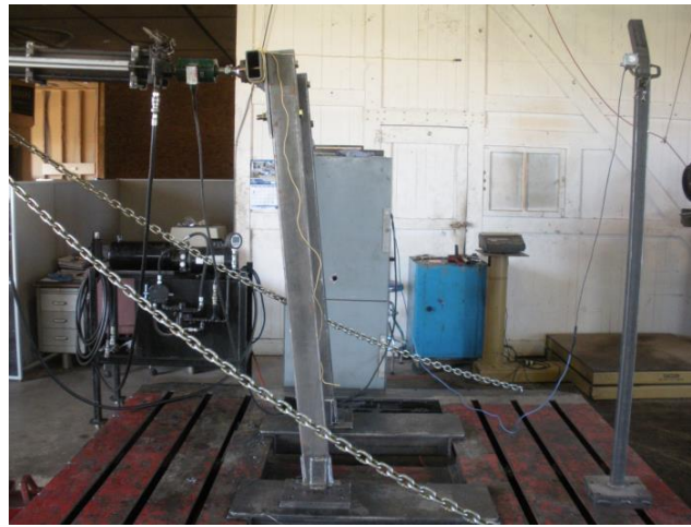
Figure 2.2. Rear load test Long 460 ROPS.
