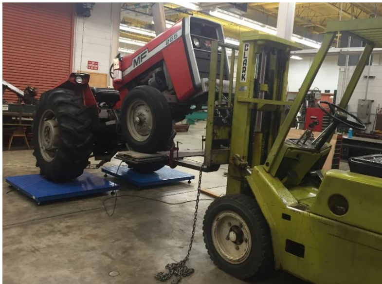
Figure 4.8. Tractor CG height measurement by using a fork lift.
