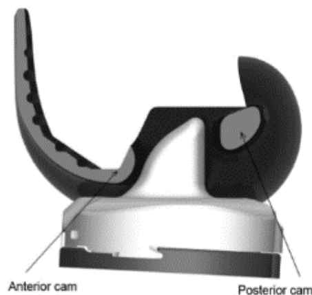
Figure 2 The journey (Smith and Nephew, Memphis, TN) bi-cruciate stabilized total knee replacement showing the anterior and posterior cams of the femoral component, and the post on the tibia (119).
