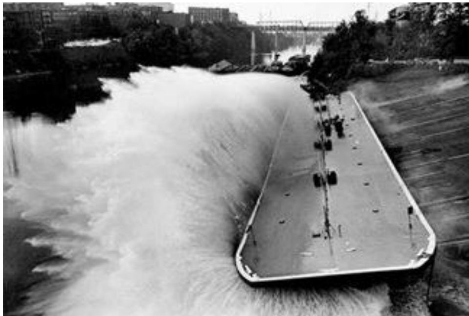
Figure 16. Barge deployment (Nashville Bridge Company).
