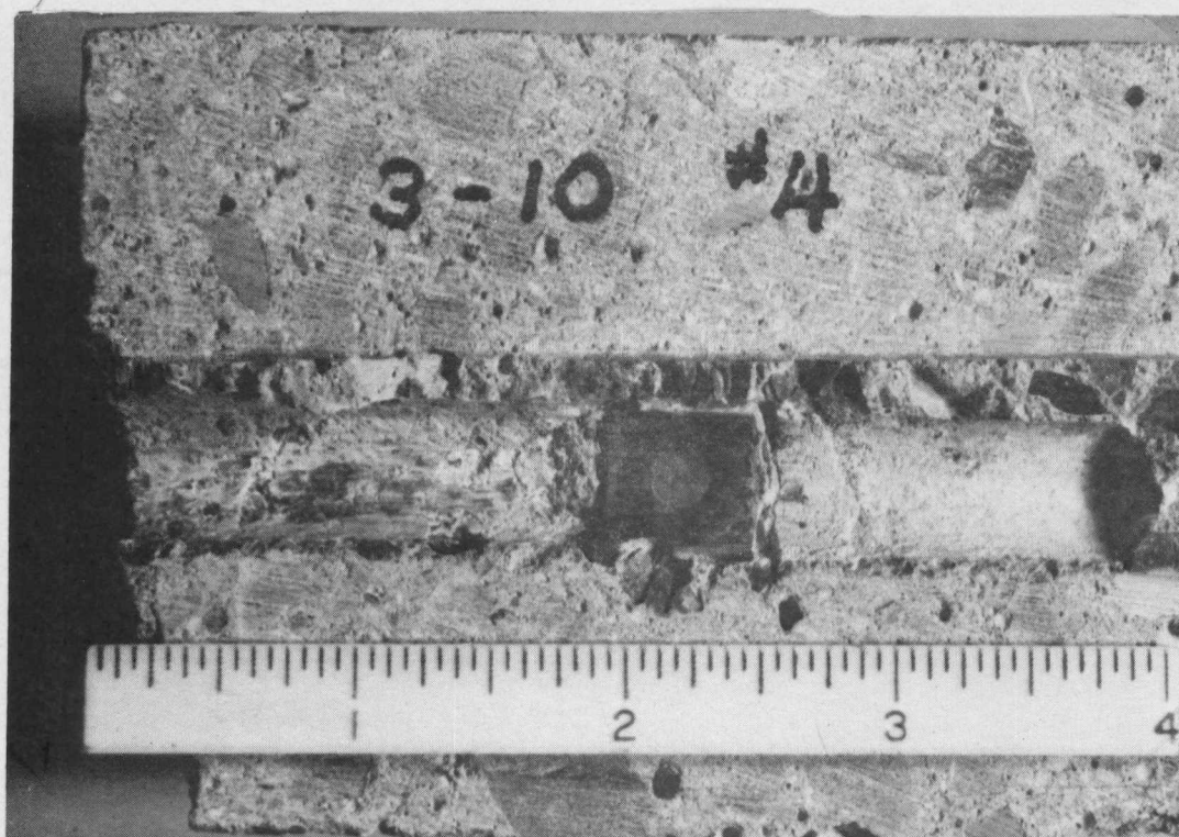
Figure 41. Closeup of 10% air content core containing wedge. Top of core is located to the left--Phase II.
