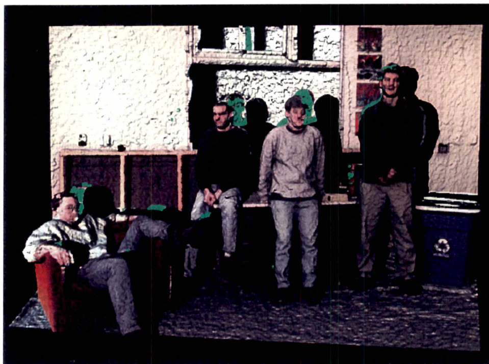
Figure 3.17: Registered color image of 'people' scene mapped onto the 2\frac{1}{2} -D model created from the range data.
