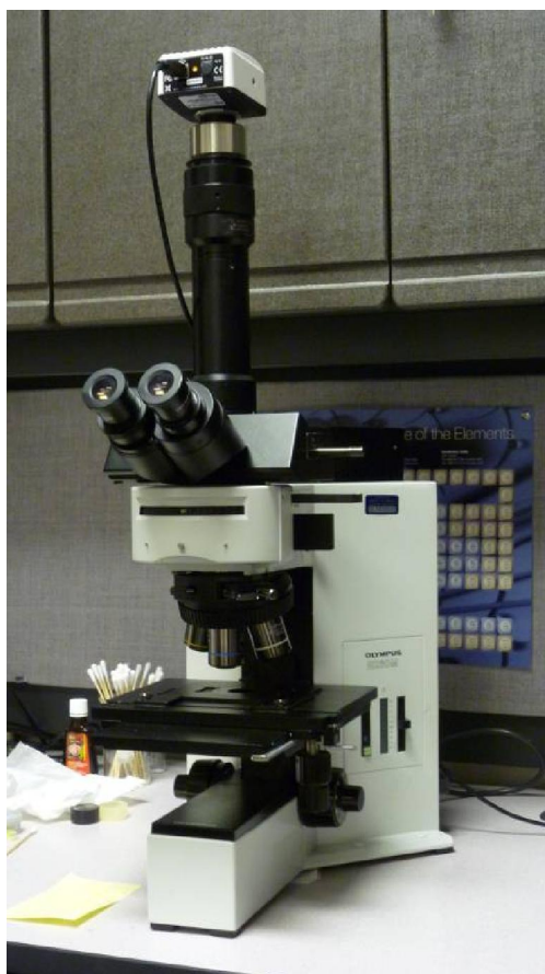
Figure 2.15 Olympus® BX60M and Infinity 1 camera
