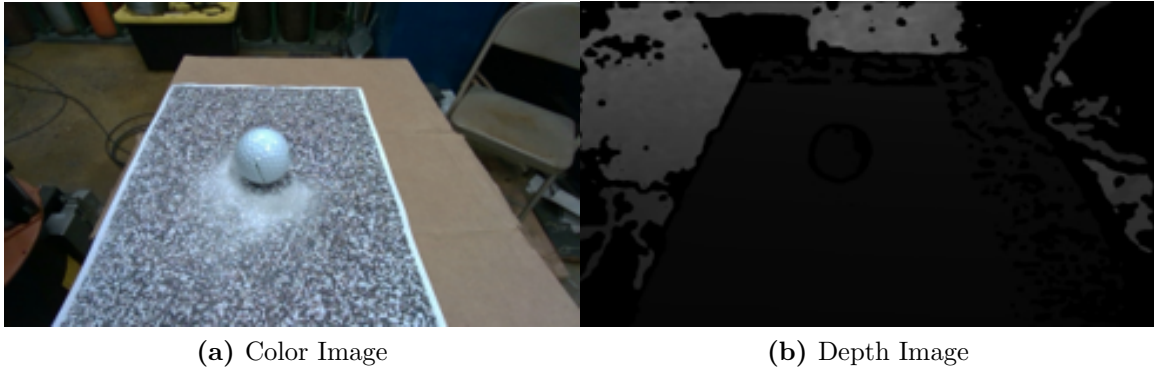
Figure 3.4: Example color and depth image from D405.
