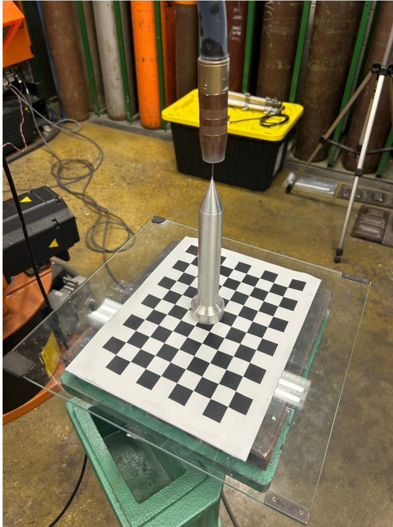
Figure 3.12: Demonstration of 4-Point touch method with the calibration. spire
