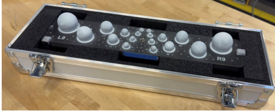
Figure 5.1: GOM PSA400 calibration artifact sprayed with titanium dioxide powder [3].
