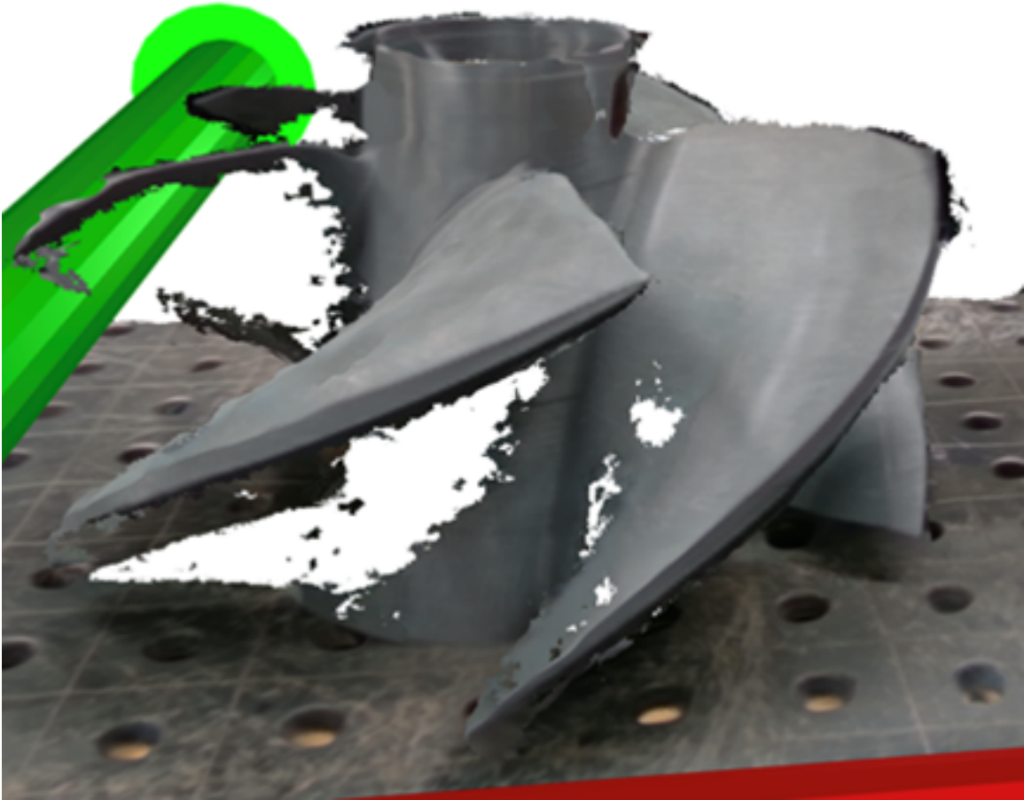
Figure 3.15: FDM propeller mesh after time and spatial synchronization.
