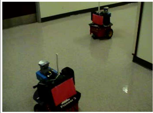
(d) Follower robot follows the red blob in the door and stops.
