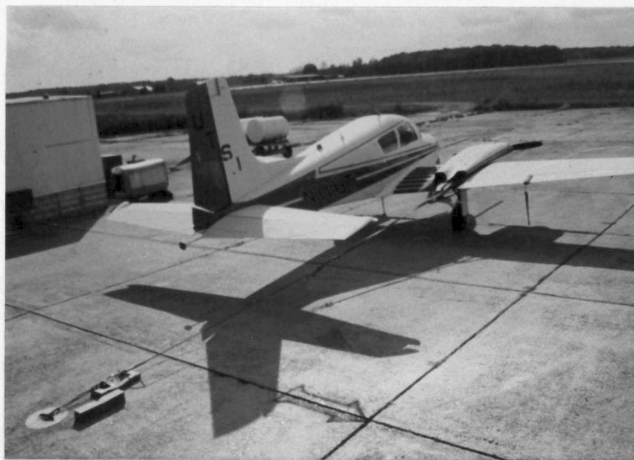
Figure 9. Static Thrust Test Setup. Dynamometer and tie-down are located in lower left corner.
