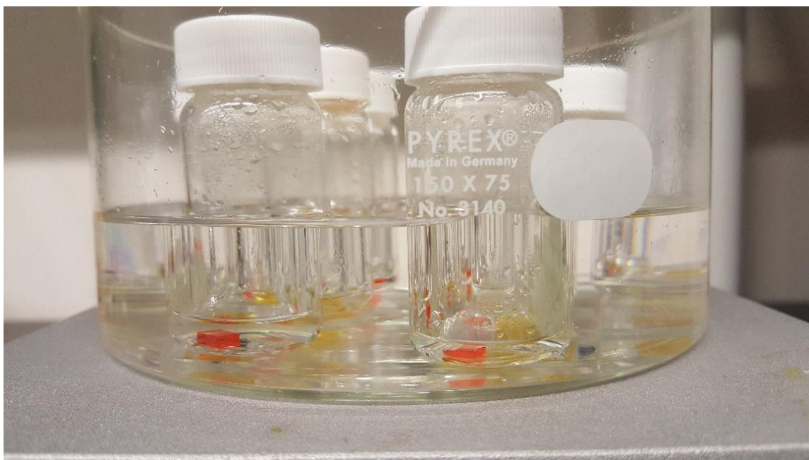
Figure 3.1. Picture showing the growth process via inverse temperature crystallization.
