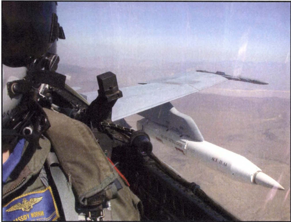
Figure 4: ACE pod used for captive AMRAAM testing
