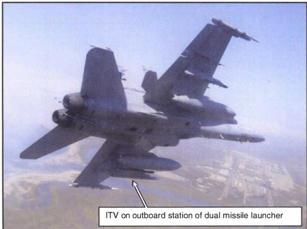
Figure 5: ITV pod used for captive AMRAAM testing
