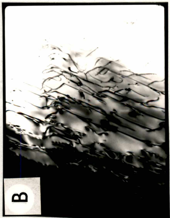
Figure 12. Transmission electron micrographs of McKinney. (A) displaying complex character of dislocations; (B) loops and jogs indicating moderate recovery of the sample; (C) subgrains imprinted with dislocations of complex character. The scale for each photomicrograph is 25\mu\text{m} = 1 \text{ micron} .
