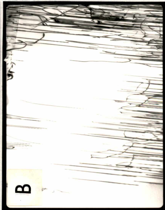
Figure 13. Transmission electron micrographs of Adrian. (A) displaying simple, straight character of dislocations; (B) heterogeneous distribution of dislocation density, ranging from 10+7 lines per square centimeter in the center to 5 \times 10+9 lines per square centimeter on the far right side of the photomicrograph; (C) heterogeneous distribution of dislocations between in smaller subgrains. The scale for each photomicrograph is 17\text{mm} = 1 \text{ micron} .
