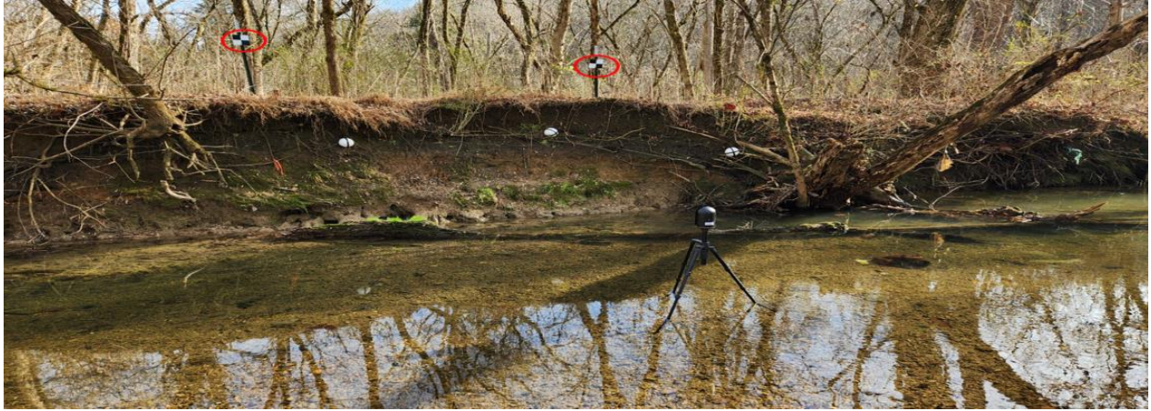
Figure 5: Photo of a regular field setup with georeferenced targets circled in red.
