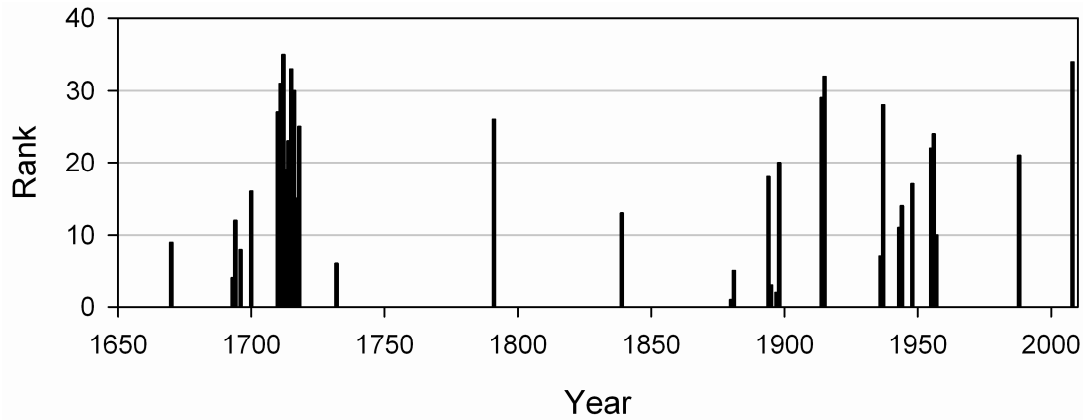
Figure 27: Valley River 5-year averages distribution of reconstructed values within the lowest 10th percentile. The y-axis represents the rank for the period of low flow, and the x-axis represents the end year for the 5-year average period of the reconstructed (1656–1918) and instrumental (1919–2008) record.
