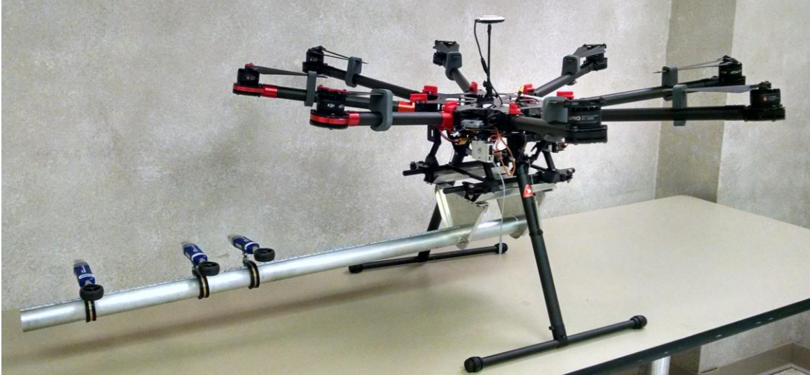
Figure 7 Drone with boom assembly and anemometers
