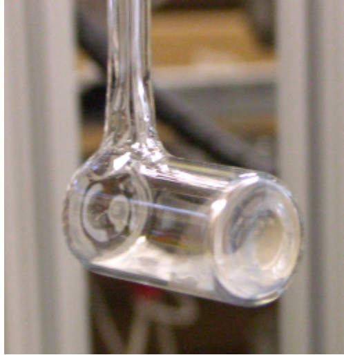
Figure 3.1: A picture of the ^3\text{He} analyzer cell, connected to the filling station at the SNS.
