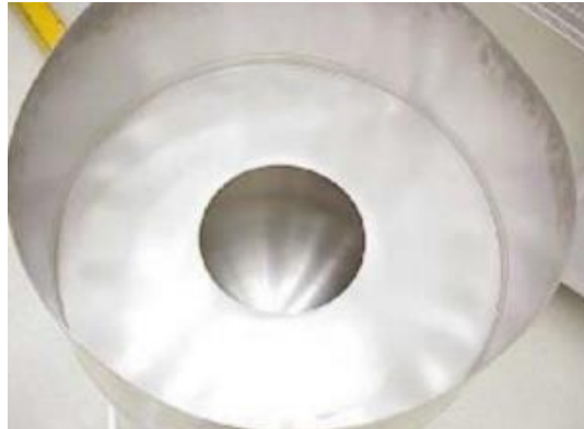
Figure 2.7 – Circular baffle welded to the interior of a tank [29].
