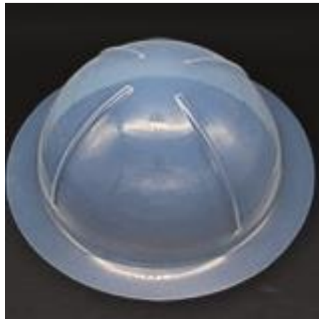
Figure 5.10 – Hemispherical FEP diaphragm tank [65].
