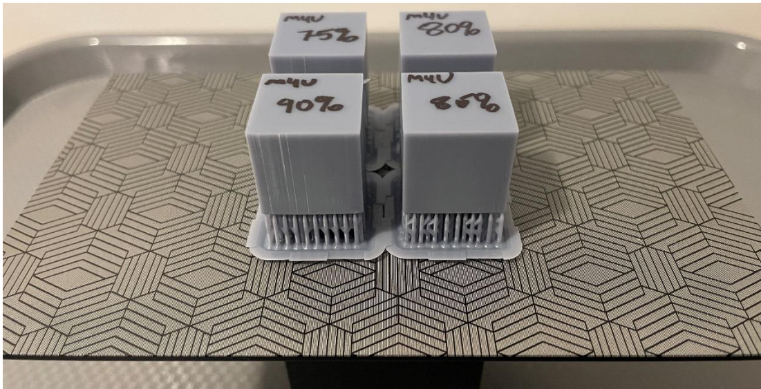
Figure 5.23 – M4U support density cube print.
