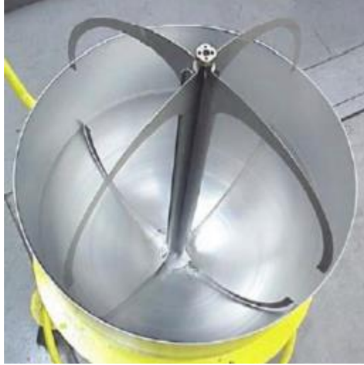
Figure 2.9 – Total-communication vane PMD [29].
