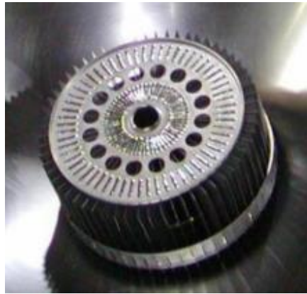
Figure 2.12 – Sponge PMD for a cesium propellant ion engine [29].
