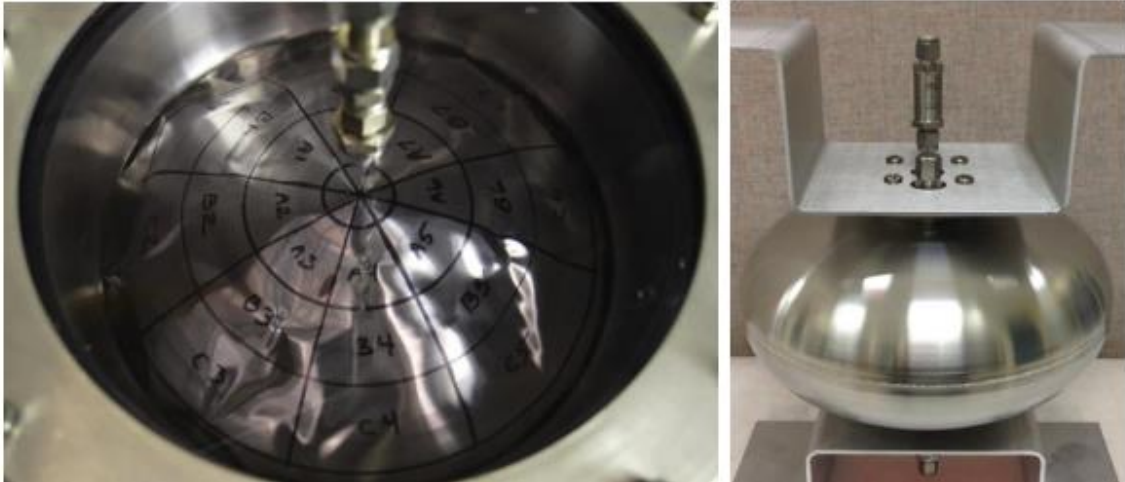
Figure 2.4 – NASA JPL's diaphragm tank for Busek's CMNTs [31].
