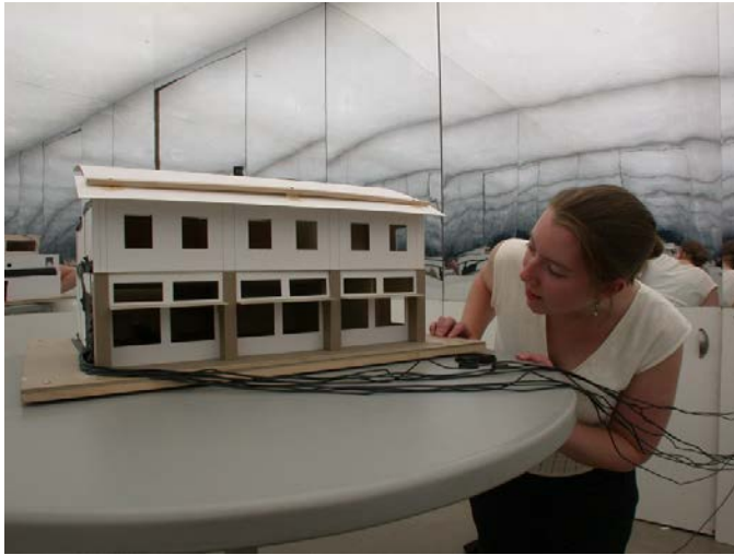
Figure 7. Daylight study at PEC lab
