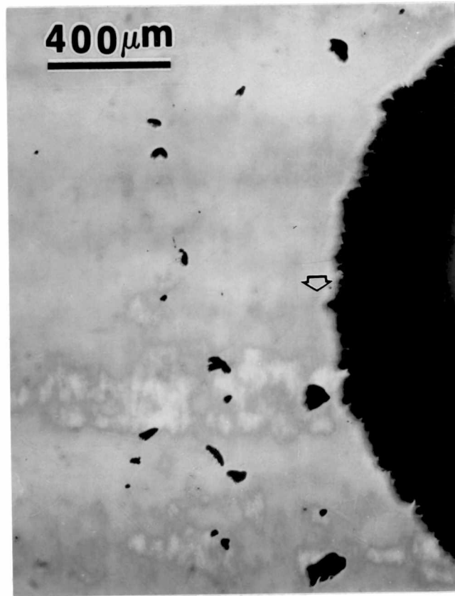
Figure 4.2-10 A Blunted Precrack and Creep Cavitation in the Creep Zone at the Crack Tip (The Arrow Indicates the Location of the Crack Tip as Shown in Figure 4.2-8)
