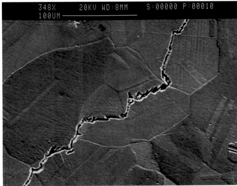
Figure 4.2-9 A Precrack Produced by Fatigue at Room Temperature Showing the Remaining Crack Tip Damage Along the Crack Sides
