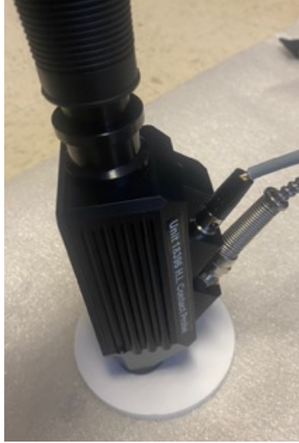
Figure 3.3: Contact probe making contact with the Spectralon panel. This is to collect a white reference.
