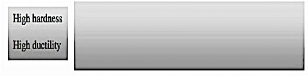
Figure 1. Cross-section of a FGAC. Adapted from [20] illustrating the variation in properties from the hard front region to back ductile region achievable through PMMC technology.
