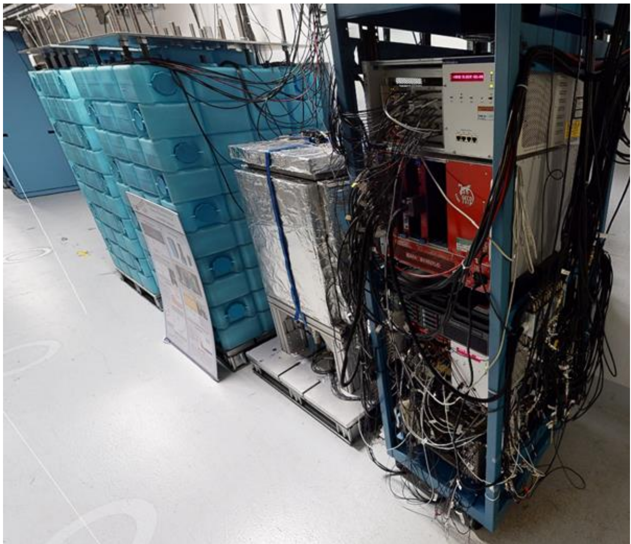
Figure 37. NUBES electronics rack with NaI detector positioned between this and the two active Neutrino Cubes on the left.
