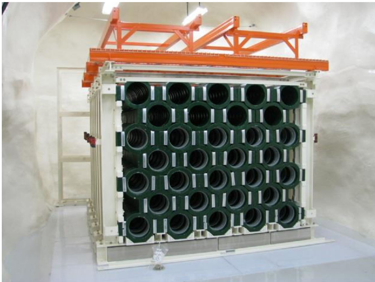
Figure 34. HALO detector in place at SNOLAB facility. The empty cavities are where the ^3\text{He} proportional counters are to be placed.
