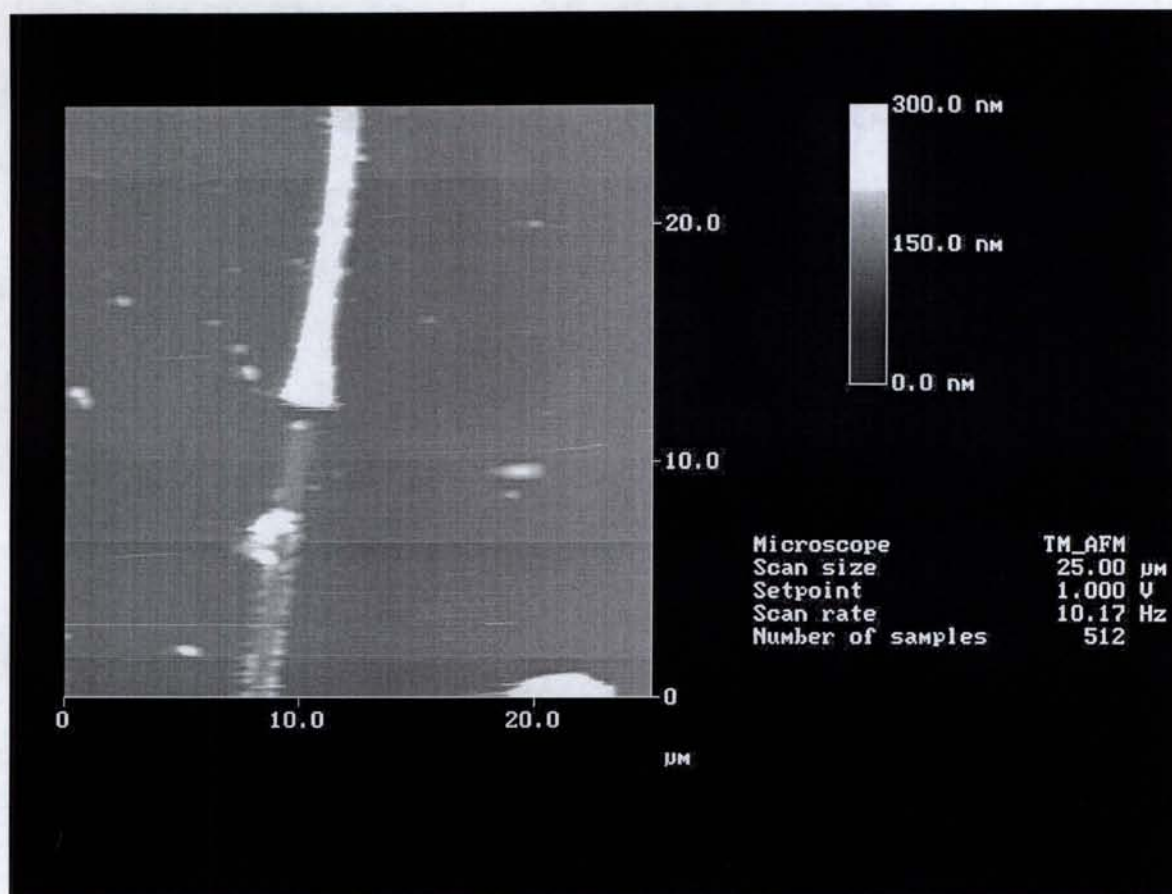
Figure 7: Condition of device #4 after multiple deposition and dissolution of Ni (top electrode negative, bottom electrode ground)
