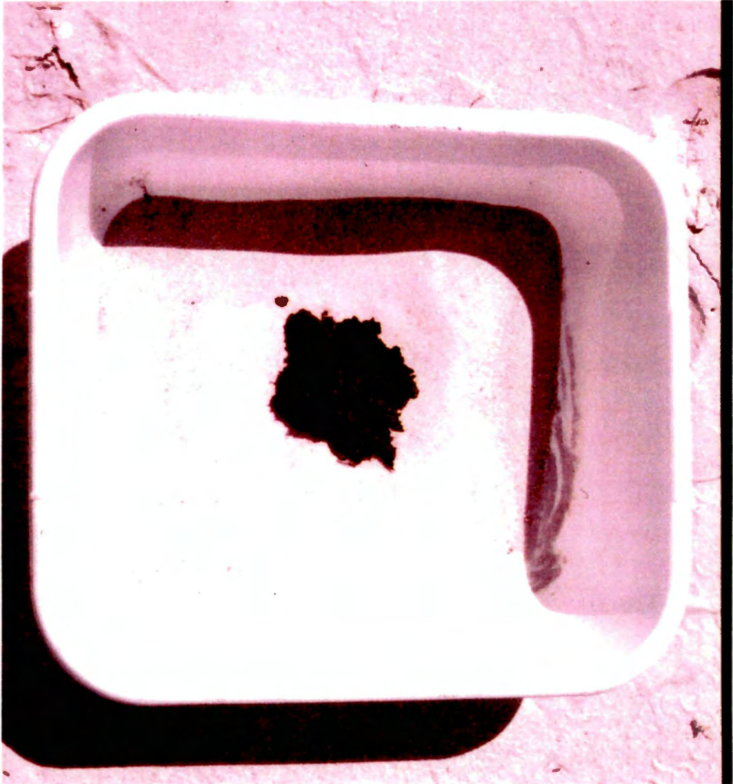
Figure 2.1. Cow pat in pan. 150 gram manure pat on sand inside a white plastic dishpan placed on the experimental sand bed.
