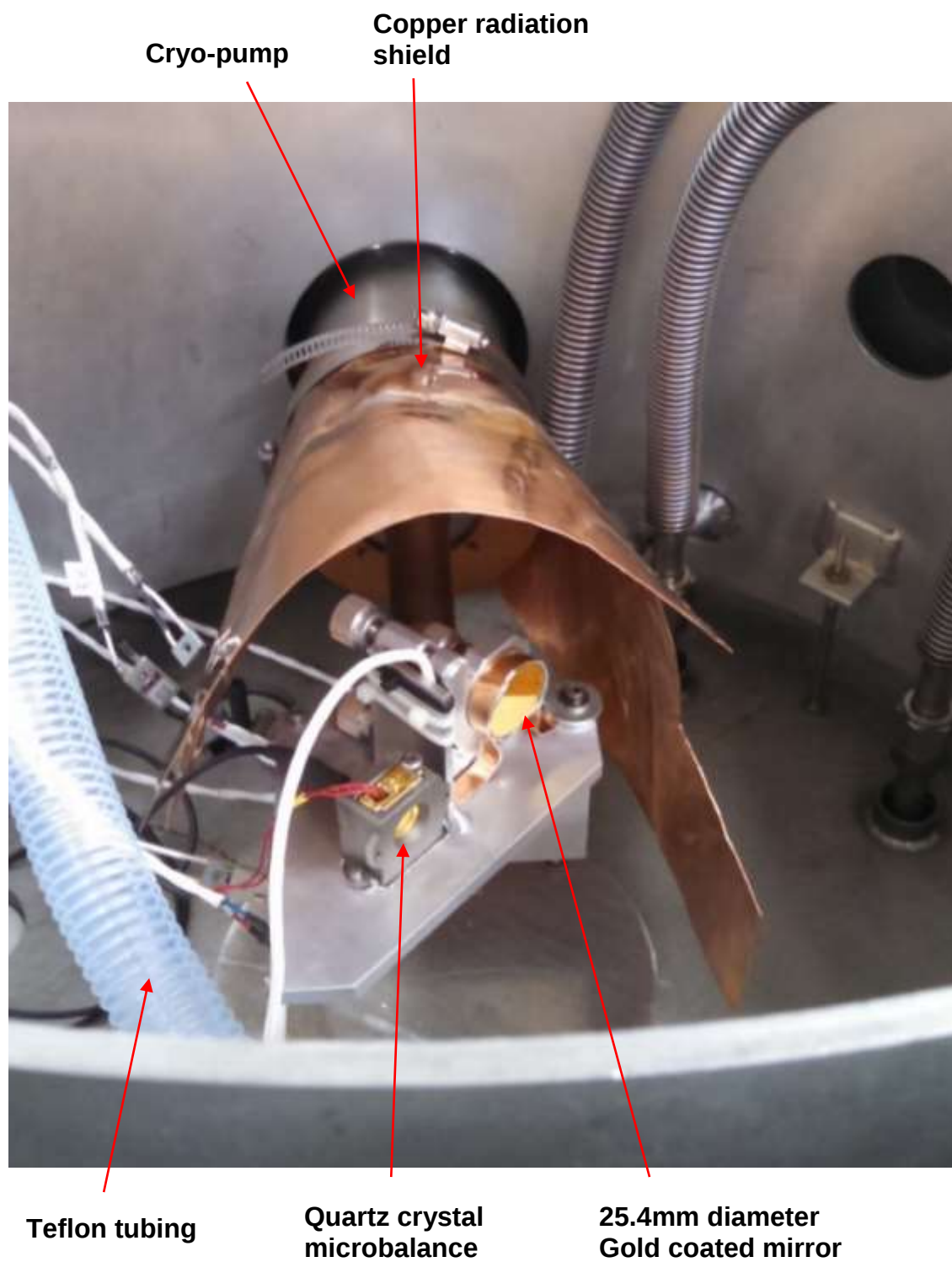
Figure 2.9: Interior chamber components.
