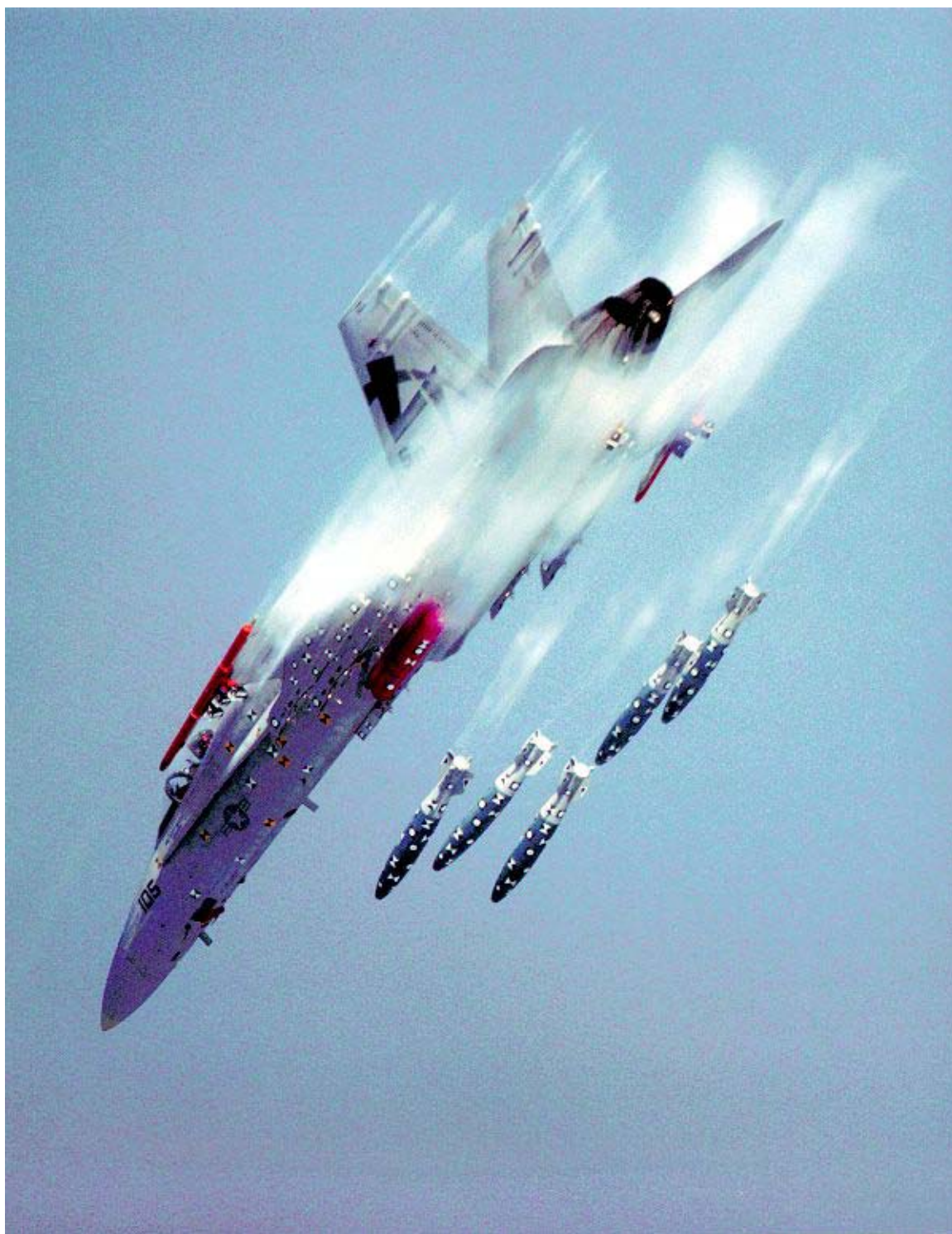
Figure 1 F/A-18A HORNET PERFORMING SAFE SEPARATION TESTING Photo courtesy Vernon Pugh
