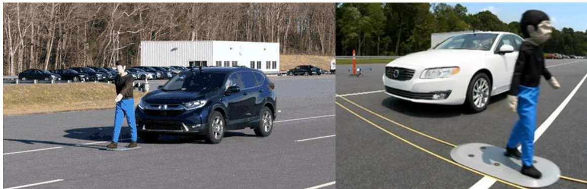
Figure 5-2 IIHS Pedestrian Crash Prevention System Testing, IIHS Images (209)
