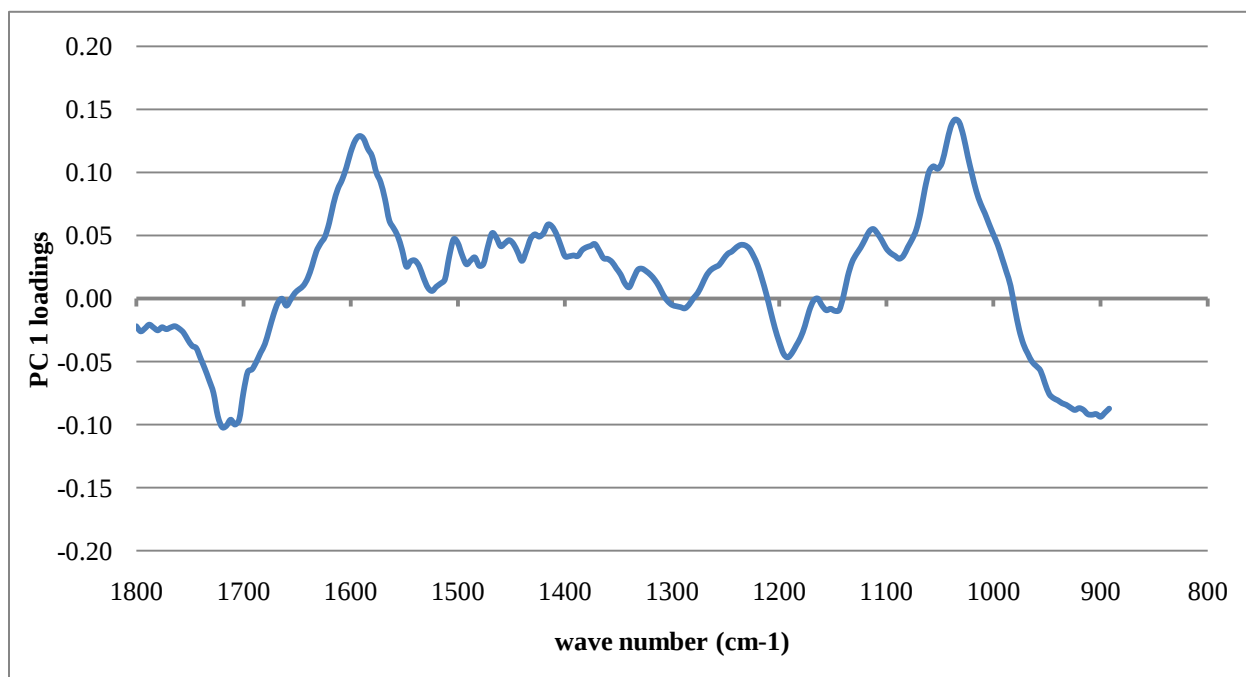
Figure 16: PC1 loadings plot for PCA of irradiated maple veneers, with 5 kGy samples withheld from analysis.
