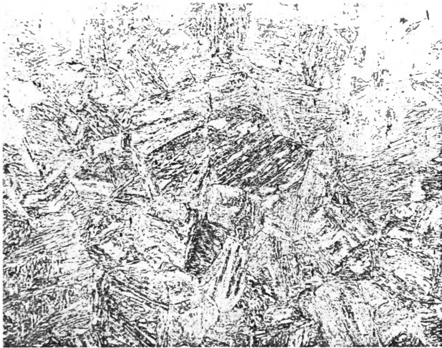
Figure 36. Photomicrograph of Climax 3Cr-1.5Mo Gleeble specimen, 35 KJ/in (1.38 KJ/mm). OLM. 200X. Nital-Picral.
