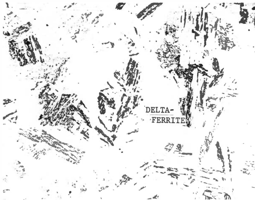
Figure 31. Photomicrograph of 9Cr-2Mo Gleeble specimen, 150 KJ/in (5.91 KJ/mm). OLM. 200X. HCl-Picral.
