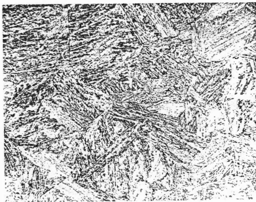
Figure 39. Photomicrograph of Lukens 2 1/4Cr-1Mo-0.12C Gleeble specimen, 150 KJ/in (5.91 KJ/mm). OLM. 200X. Nital-Picral.
