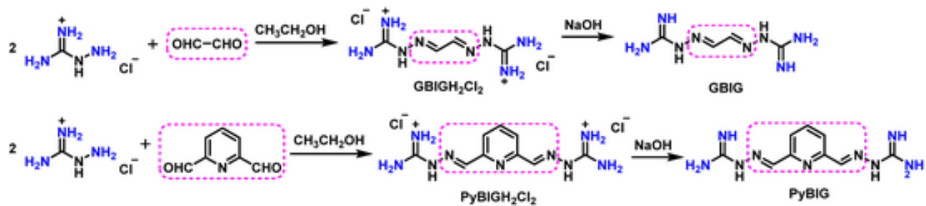
Figure 1.4 Representative procedures for the synthesis of iminoguanidine-derived sorbents
