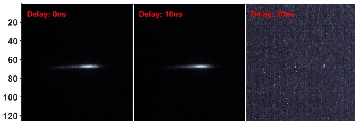
Figure 5.5 \text{N}_2^+ photoemission delay study showing short lifetimes of first negative band contributions.
