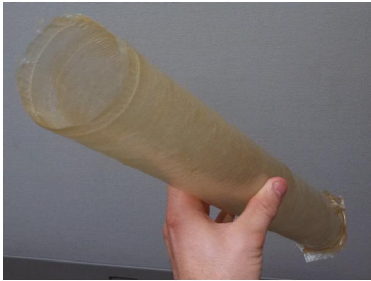
Figure 9: Fiberglass tube liner which provided a smooth internal flow path for the ISW and TCS tests.
