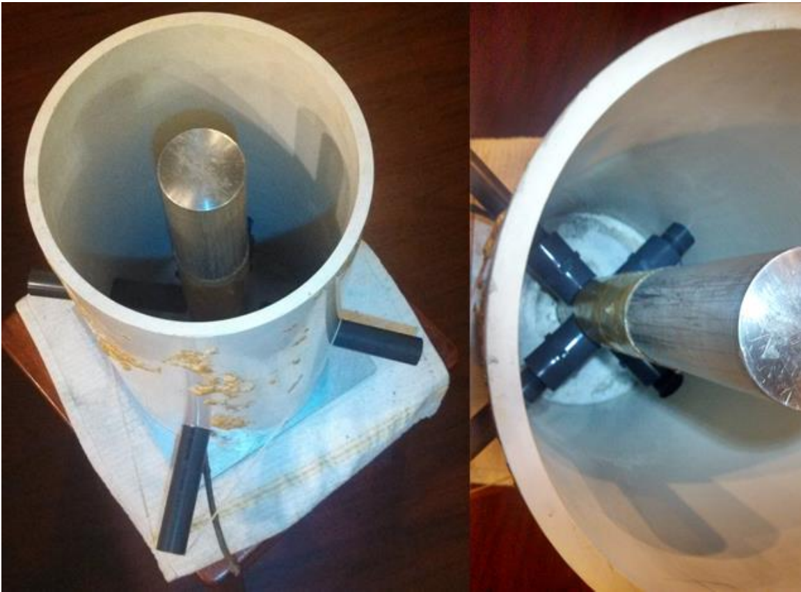
Figure 12: Mold prepared to form insulation around the ISW model vents.
