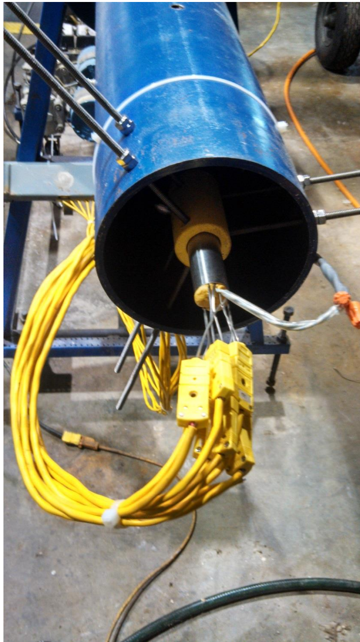
Figure 4: ESW model installed in the 15.24 cm blowdown wind tunnel.
